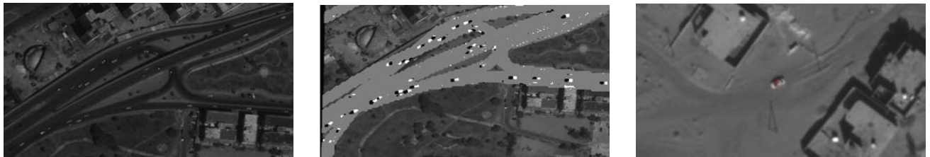
Figure 1: Left: Panchromatic WorldView-2 image of a city with traffic activity. Centre: After the roads have been extracted, PCA produces an output image in which neighbouring dark and bright polygons are visible, an indication of moving vehicles. Right: WorldView-3 image of a rural area showing the detection of a moving vehicle on a dirt road using the same methodology.
